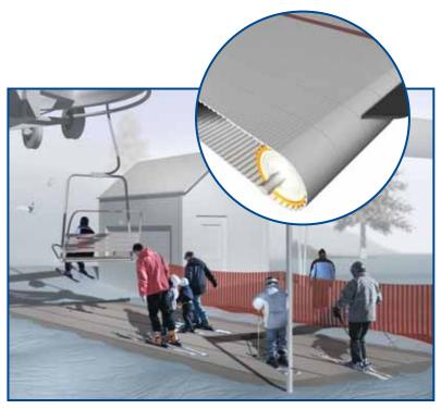
Four 450 mm wide, timing belts accelerate skiers for faster loading of detachable chair lifts. Timing belts ensure uniform speed of each skier.
