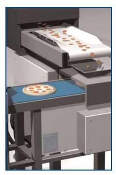
CenterClean belts are constructed with flexible urethane and sealed Kevlar tension members. This construction allows CenterClean belts to be troughed or run on small diameter pulleys with minimal belt stretch.
